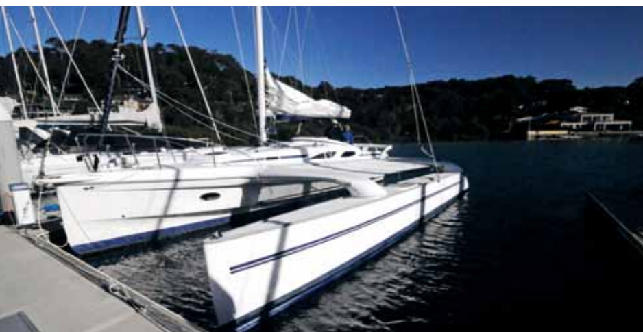
Top down: Easy as one, two, three... the Dragonfly 35 extends her floats. Folded in means this multihull can be berthed in a monohull-size pen.
